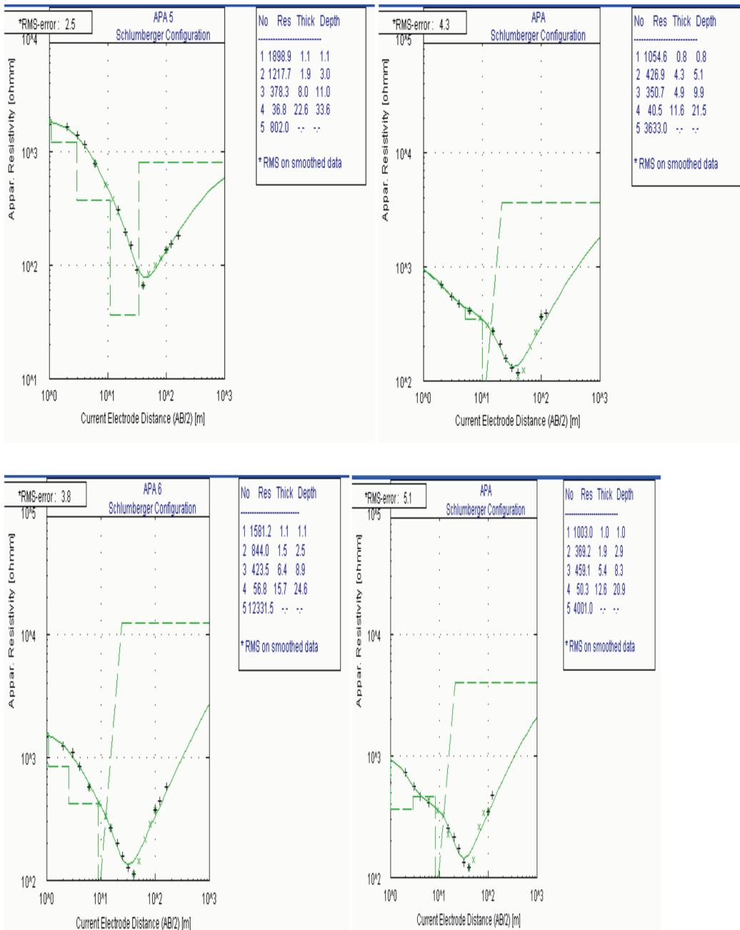
Fig.2b: Observed,Computed VES Points(5-8) and Layered Inversion Model
